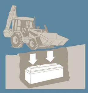
A vault protects the casket from the downward pressure in addition to the already present soil pressure.
