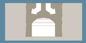
Trigard's "down and out" cover design helps distribute the continuous downward force of the soil to the vault's perimeter for a better seal and better casket protection.
